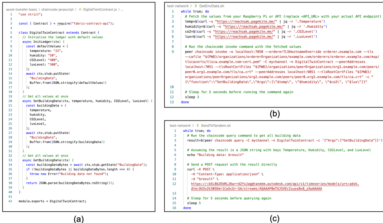
Figure 7. a) Chaincode for digital twin b) Bash script for data query c) Bash Script for data synchronization with the digital twin platform
